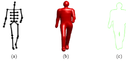
Fig. 1. (a) The 3D human skeleton model. (b) The 3D human convolution surface model. (c) The 2D convolution curves.
